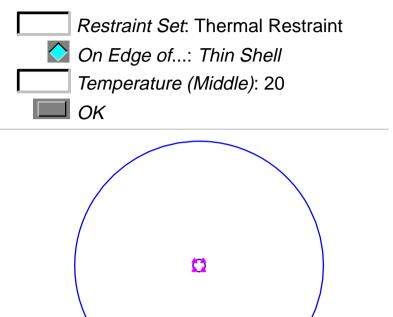
Why: The blade is bolted tightly to a solid shaft which will conduct heat from the blade. This is modeled as a temperature restraint.
