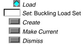
Why: A load set is required for buckling, even though no loads will be supplied in addition to the thermal load set.
